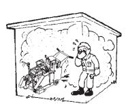
narrow area where free flow of the air is restricted. If the air flow is restricted it will cause serious damage to the saw's engine and may cause injury to people. Remember the saw's engine gives off **DEADLY** carbon monoxide gas.
